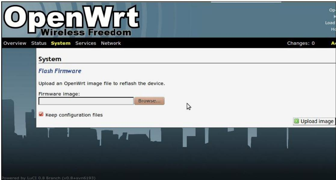
When the file has been uploaded, the **Checksum** and **Size** details will be displayed. Click on the **Proceed** button and the flashing process will begin. This may take several minutes and then the MP device will restart.
