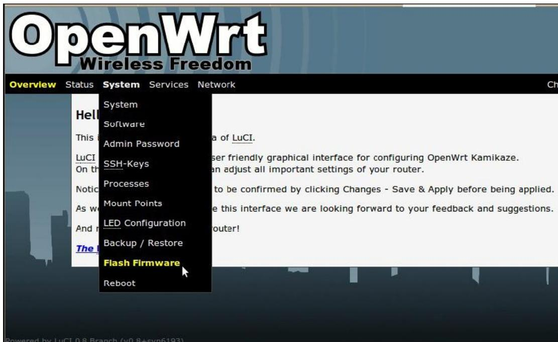
When the **Flash Firmware** page appears, click on the **Browse** button and select the required .img file from your PC file system. Then click on the **Upload image** button. The firmware will be loaded into MP via the web browser.
