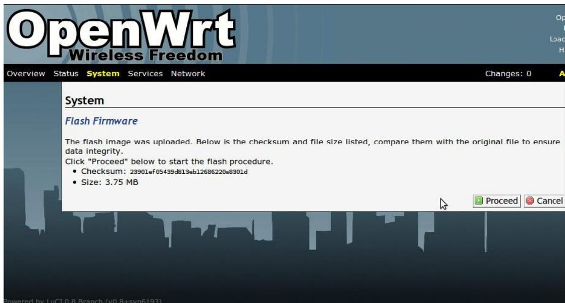
After the MP device has restarted and the WiFi led has started to flash, allow three minutes for the flashing process to complete. After that you should be able to connect to the MP device with web browser or telnet on the default LAN or Fallback IP addresses.
