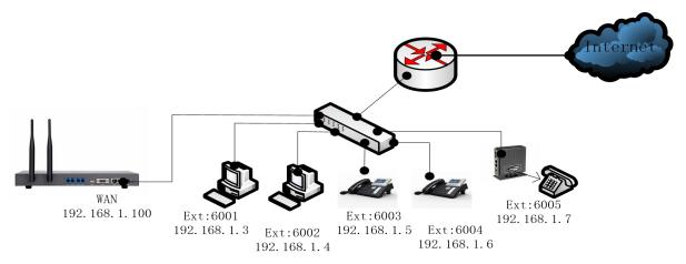
**NOTE**: It's recommended to re-set IP address of IPPBX via WAN at the first time, Since DHCP server on LAN port is enabled by default, Other DHCP client enabled devices in the network may obtain IP from IPPBX rather than real DHCP server. And then access IPPBX via LAN after configuring LAN settings.
