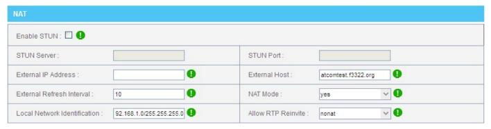
The External IP, External Host and Local Network Identification settings are used if you use IPPBX behind a NAT device to communicate with services on the outside.
