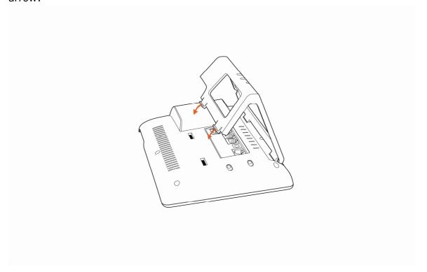
C. It is the right picture after fixing the stand bracket below:
